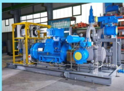
Multiphase Pump L4MG-200 388 m 3 /h @ 24 bar
