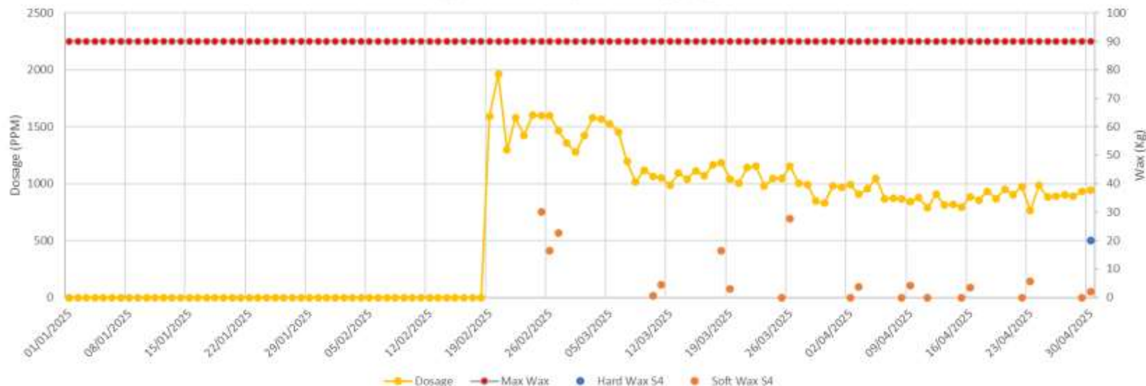
Wax Appearance Analysis from Pigging South
